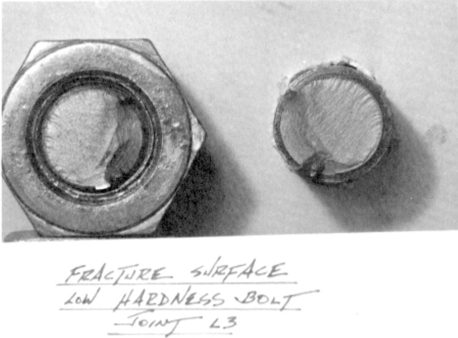
**Fig. 2.7.** Typical fatigue fracture surface.
