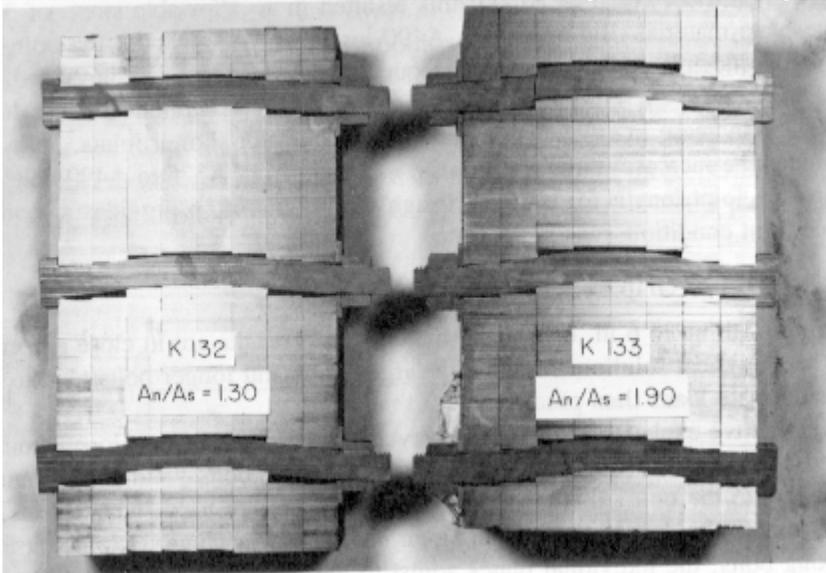
**Fig. 5.33.** Sawed sections of joints showing bolt bending.
