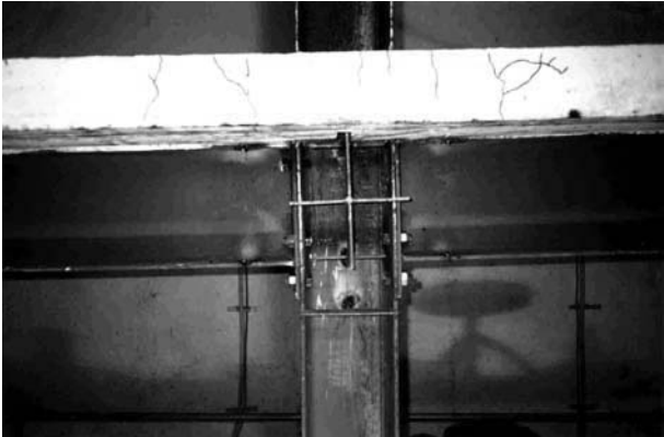
Figure 8 - Hysteresis loops and failure mode of an internal node with a steel column.
