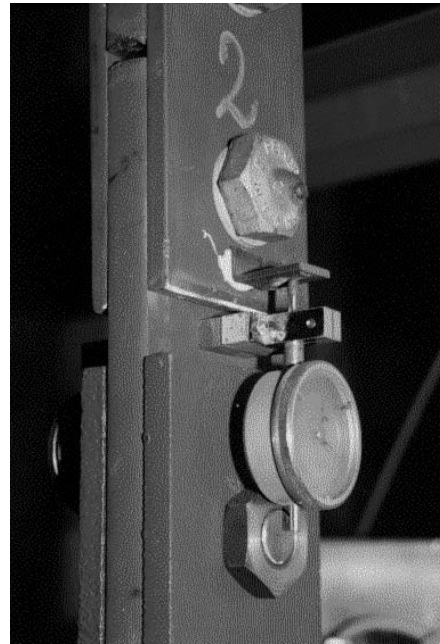
Figure 7. Measurement of displacements. Each test specimen contains two bolts, so that a total of 8 bolted connections were tested. The displacements at each bolt are measured at the head and at the nut side.
