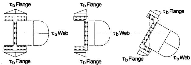
(b) Shear Stresses Due to Beam Action  $\tau_b = \frac{VQ}{It}$
